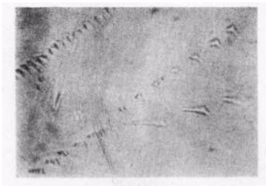
图 9 (111)面上的蚀斑三叉亚晶界  $\times 1200$
