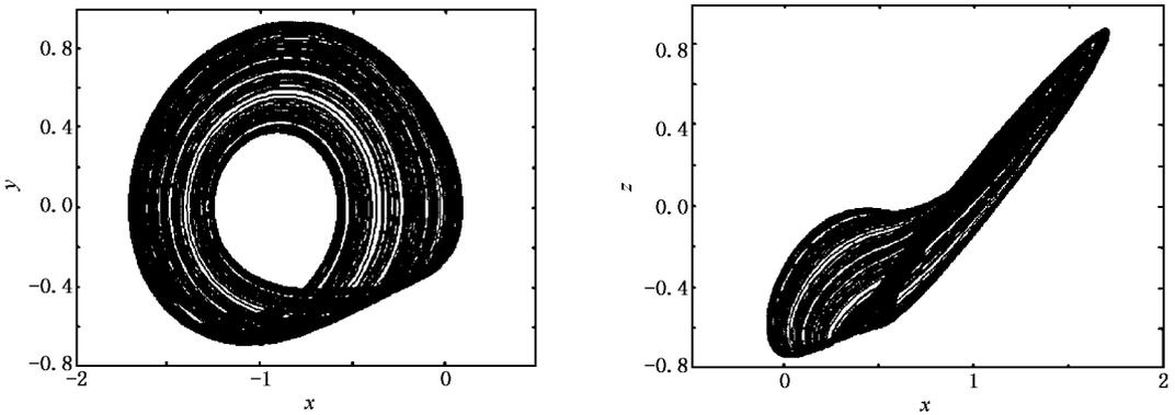
图 9 单层单螺旋混沌吸引子( $\alpha = 0.52$ ,  $\lambda_{\max} = 0.0761$ )
