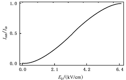
图4  $\theta = 0.229\pi, \varphi = 0.01\pi, L = 2.43\text{cm}, \alpha = 0.76\pi, \psi = 0.03\pi$  时,出射光强与入射光强的比值随外加电场  $E_0$  的变化曲线
