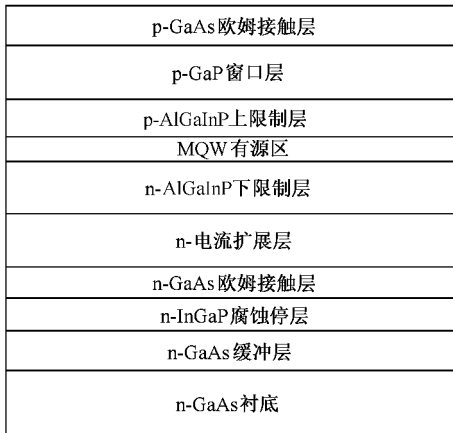
图2 AlGaInP 薄膜 LED 外延结构
