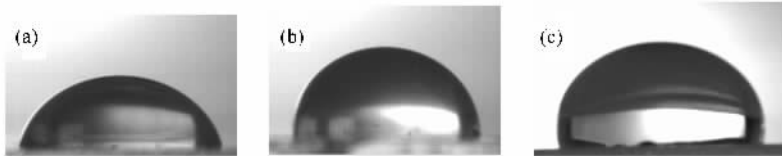
图 1 不同样品表面形成的接触角 (a)DLC (b)FN-DLC(150 W, 200℃, r = 0.75 ) (c)FN-DLC(100 W, 100℃, r = 0.75 )
