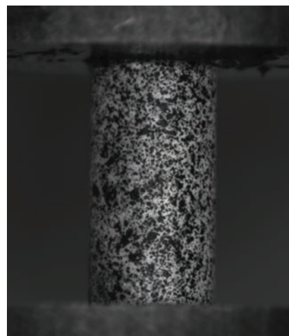
图3 喷涂了散斑点的试样照片 Fig. 3. Surface speckle image of PZT95/5 specimen.
