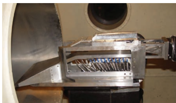
Fig. 23. Direct-connect supersonic wind tunnel with isolator model [33,44,46,66] .
