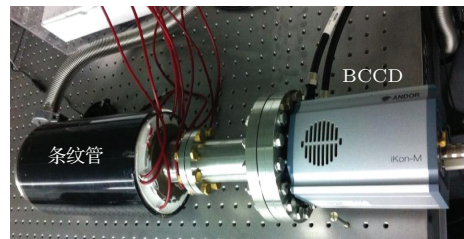
图 4 基于 EBCCD 的大动态条纹相机实物图 Fig. 4. Material object of large dynamic range streak camera based on EBCCD.
