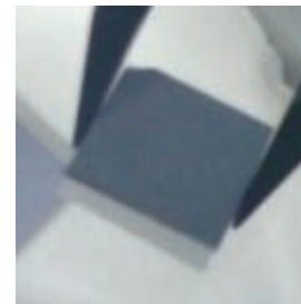
图 15 低温 GaAs 键合聚合物基底 Fig. 15. The bonding of LT-GaAs epilayers on the copolymer substrate.
