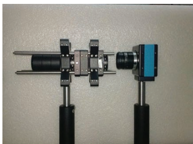
图8 (网刊彩色) 通道调制型偏振干涉成像装置 Fig. 8. (color online) Channel modulated polarization interference imager.
