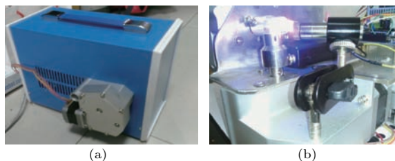
图 9 (网刊彩色) 用长余辉材料显示的激光书写样机 (a) 样机外壳; (b) 内部结构 Fig. 9. (color online) Prototype of laser writing based on the LLP material display: (a) Outer of the prototype; (b) inter of the prototype.
