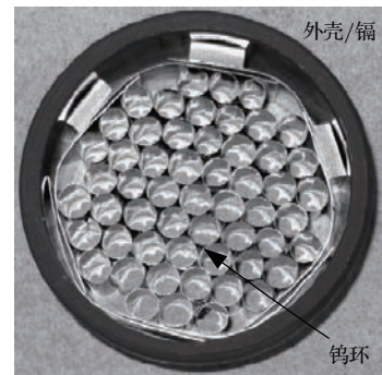
图8 PULSTAR源环状钨靶/慢化体照片 Fig. 8. Photograph of converter/moderator bank used in the PULSTAR positron source.
