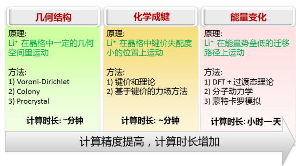
图 3 计算离子输运性质的几类方法及对应的计算量 Fig. 3. The calculation methods for ion conduction and the computation costs.
