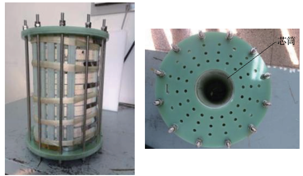
图 5 采用第二代高温超导带材绕制的磁体实物图 Fig. 5. The picture of high-temperature superconducting magnet using by YBCO tapes.
