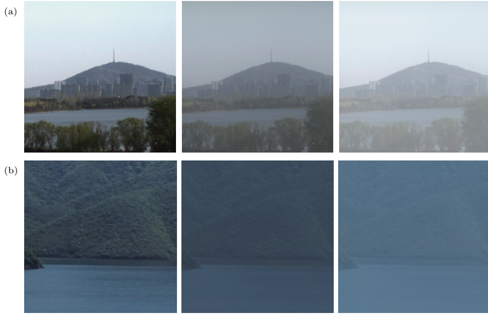
图7 实际场景仿真 原场景图(左); M_{TF} 影响的场景图(中); M'_{TF} 影响的场景图(右); (a) \tau = 0.30, g = 0.9, \bar{\varpi} = 0.95 ; (b) \tau = 0.35, g = 0.65, \bar{\varpi} = 0.90
