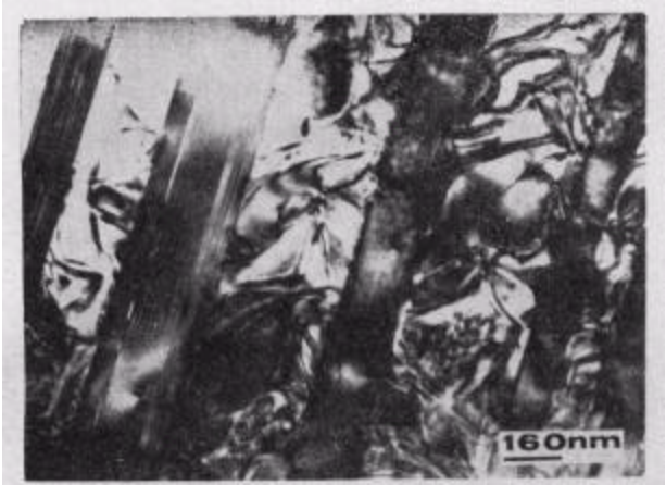
图1 铸态 \text{Ni}_3(\text{Ti}_{0.5}, \text{V}_{0.5}) 合金电子显微象
