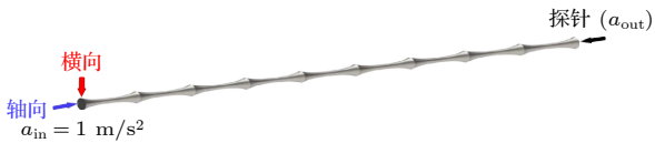
图 3 振动传输频率响应函数的有限元计算方法 Fig. 3. Finite element calculation method of the vibration transmission frequency response function.
