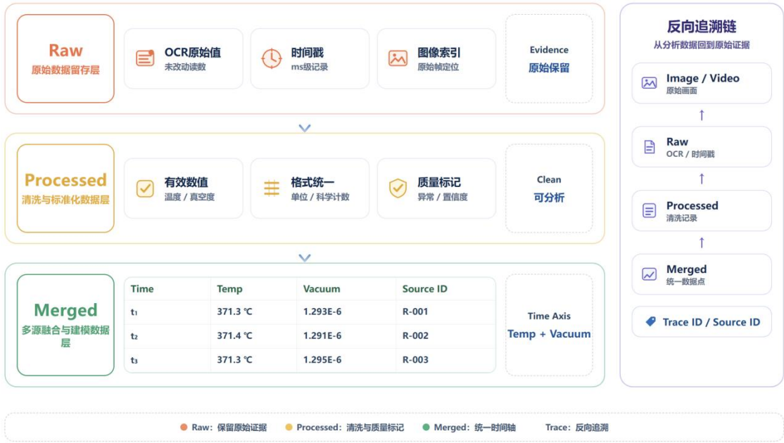
图 5 Raw-Processed-Merged 三层数据关联图谱
