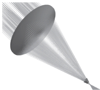
图4 二次聚光棱镜光线跟踪模拟示意图 Fig. 4. Light tracing simulation diagram under secondary condensing prism.
