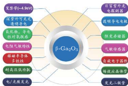
图4 \beta\text{-Ga}_2\text{O}_3 材料具有的物理性质及其对应的器件应用 Fig. 4. Physical properties and device applications of \beta\text{-Ga}_2\text{O}_3 material.
