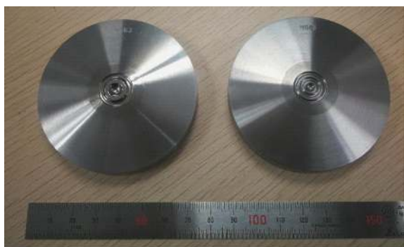
图 4 单凹曲面压砧 (左) 与双凹曲面压砧 (右) 实物图 Fig. 4. The single toroidal anvil (left) and double toroidal anvil (right).
