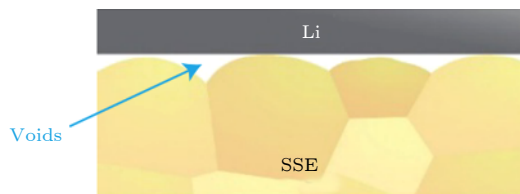
图 4 无机固态电解质与锂负极之间的“点对点”式接触 [16] Fig. 4. Point-to-point contact between the inorganic solid state electrolyte and Li anode [16] .
