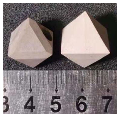
图 3 磨倒棱 (左) 和未磨倒棱的八面体 (右) Fig. 3. Chamfered (left) and unchamfered octahedron (right).
