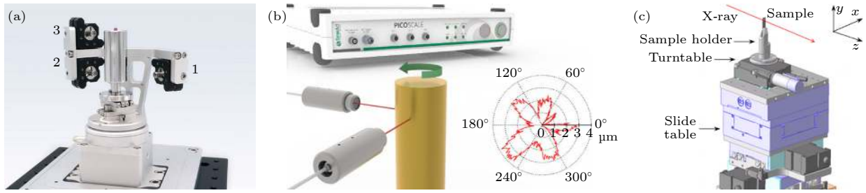
图 2 在线机械校准 (a) 激光干涉仪 [4] ; (b) 激光干涉仪记录旋转目标偏移轨迹 [4] ; (c) 上海光源软 X 光谱学显微实验站样品台 [5] Fig. 2. Online mechanical calibration: (a) Laser interferometer [4] ; (b) laser interferometer records the deviation trajectory of the rotating target [4] ; (c) SSRF soft X spectroscopy microscope experimental station sample stage [5] .
