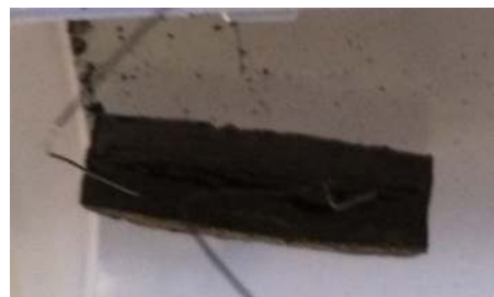
图 1 \text{Mg}(\text{BH}_4)_2 原位烧结制备的 \text{MgB}_2 块材 Fig. 1. \text{MgB}_2 bulk fabricated by in situ reaction from \text{Mg}(\text{BH}_4)_2 .
