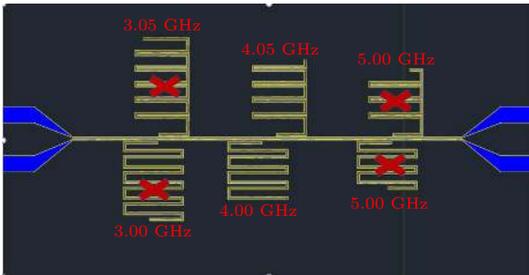
图 3 单个四分之一波长共面波导谐振器样品图,图中打红叉的谐振器已经短接 Fig. 3. Sample diagram of single quarter wavelength coplanar waveguide resonator. The resonators with the red crosses have been shorted.
