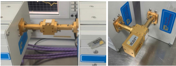
图 19 SIW-RWG 过渡结构和一分二过渡结构实测场景 Fig. 19. Measured scenes of SIW-RWG transition structure and one to two divider transition structure.
