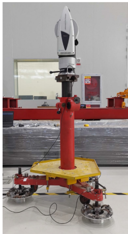
图 8 宽频隔振器长时间静态力学试验照片 Fig. 8. Photograph of long time static mechanical test of isolator with broadband characteristic.
