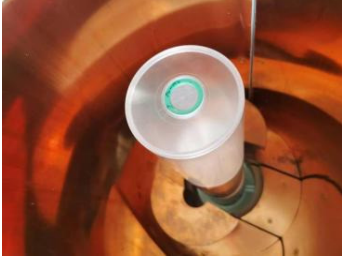
图 2 高纯锗及内部支架 (源放在支架中心处) Fig. 2. High purity germanium and internal bracket (source placed at the center of the bracket).
