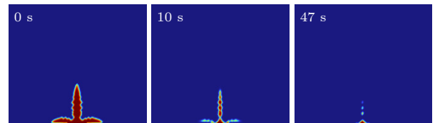
图 8 未耦合力学场、环境温度 353 K 下锂枝晶的溶解形貌 Fig. 8. Dissolution morphology of lithium dendrites at ambient temperature of 353 K in the uncoupled mechanical field.
