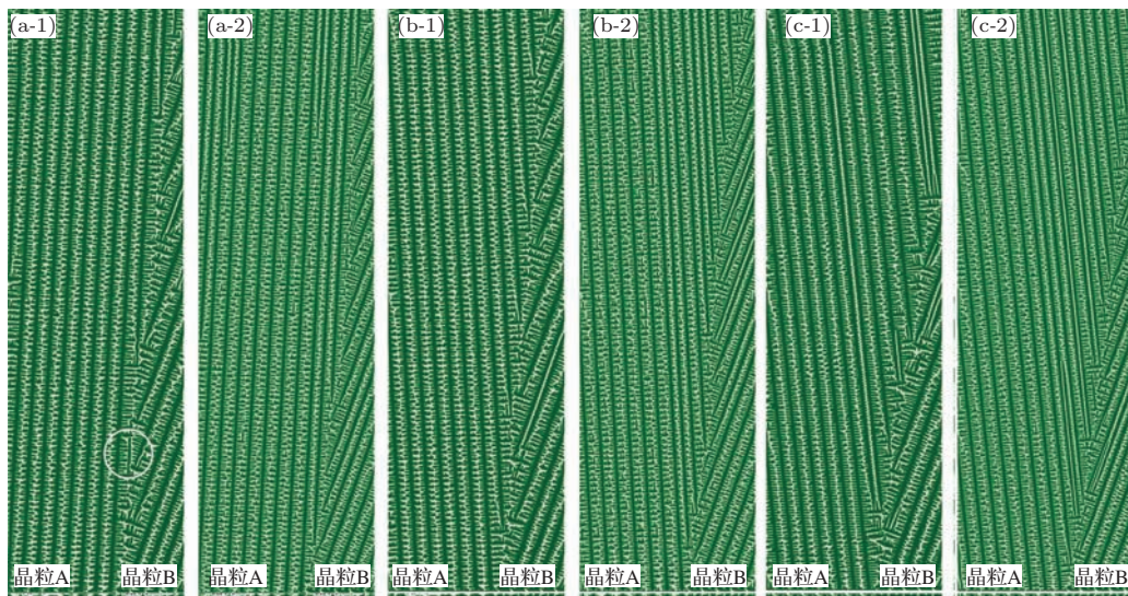
图7 不同优先生长角度和不同抽拉速度下发散双晶竞争生长模拟结果 (a-1) V = 150\text{ }\mu\text{m}\cdot\text{s}^{-1} , \theta_A = 3^\circ , \theta_B = 20^\circ ; (a-2) V = 300\text{ }\mu\text{m}\cdot\text{s}^{-1} , \theta_A = 3^\circ , \theta_B = 20^\circ ; (b-1) V = 150\text{ }\mu\text{m}\cdot\text{s}^{-1} , \theta_A = -3^\circ , \theta_B = 20^\circ ; (b-2) V = 300\text{ }\mu\text{m}\cdot\text{s}^{-1} , \theta_A = -3^\circ , \theta_B = 20^\circ ; (c-1) V = 150\text{ }\mu\text{m}\cdot\text{s}^{-1} , \theta_A = -6^\circ , \theta_B = 20^\circ ; (c-2) V = 300\text{ }\mu\text{m}\cdot\text{s}^{-1} , \theta_A = -6^\circ , \theta_B = 20^\circ
