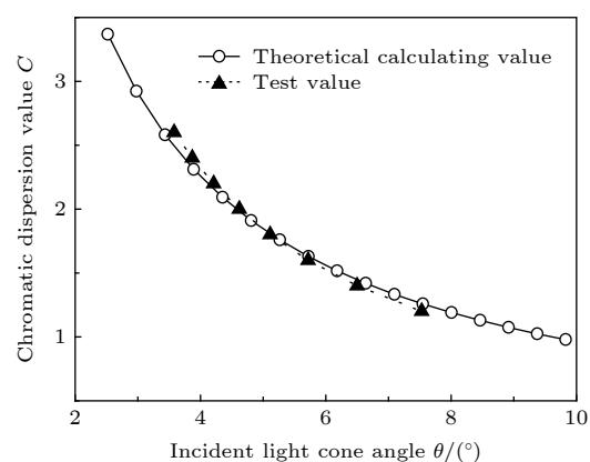
图 7 色散量  $C$  的理论值和测试值与入射光束锥角  $\theta$  关系曲线的对比Fig. 7. Contrast curves of the relationship between the test and theoretical value of  $C$  with  $\theta$ .
