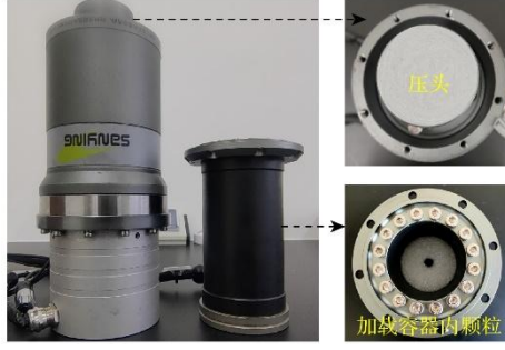
Figure 8. Indenter and specimen.
