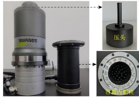
Figure 5. Indenter and specimen.
