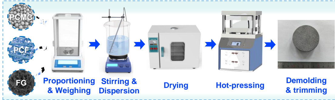
Figure 1. Flowchart of the preparation process for multidimensional carbon-based thermally enhanced microcapsule phase change composite.
