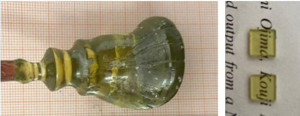
图 1 Pr, Yb, Ho: \text{GdScO}_3 晶体及切片 Fig. 1. As-grown Pr, Yb, Ho: \text{GdScO}_3 crystal and slices sample.
